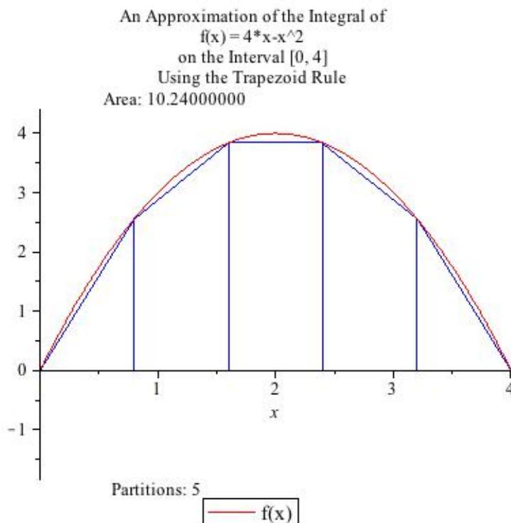
Because the tops of the slices are allowed to slant, they remain much closer to the graph  $y = f(x)$  than do the Riemann sums. Because the area of a right trapezoid is the average of the areas of the two rectangles whose heights are the value of  $f$  at the two endpoints, it is easy to compute the trapezoidal approximation: it is just the average of the left-Riemann sum and the right-Riemann sum corresponding to the same partition into vertical strips.
