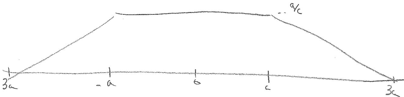
$$t = \frac{5}{2} \frac{a}{c} \quad u(x,t) = \frac{1}{2c} \text{Length} \left\{ \left( x - \frac{5}{2}a, x + \frac{5}{2}a \right) \cap (-a, a) \right\}$$
