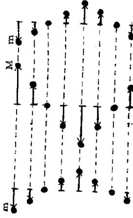
These three simple motions are called the normal modes of oscillation of the molecule. They are the oscillations determined by the  $\phi_1$ ,  $\phi_2$ , and  $\phi_3$ . Every motion of the system is a linear combination of the normal modes of oscillation, the particular oscillation depending on what initial conditions are given. By an appropriate choice of the initial conditions, one or another of the normal modes will result. Otherwise some less recognizable motion will result.
