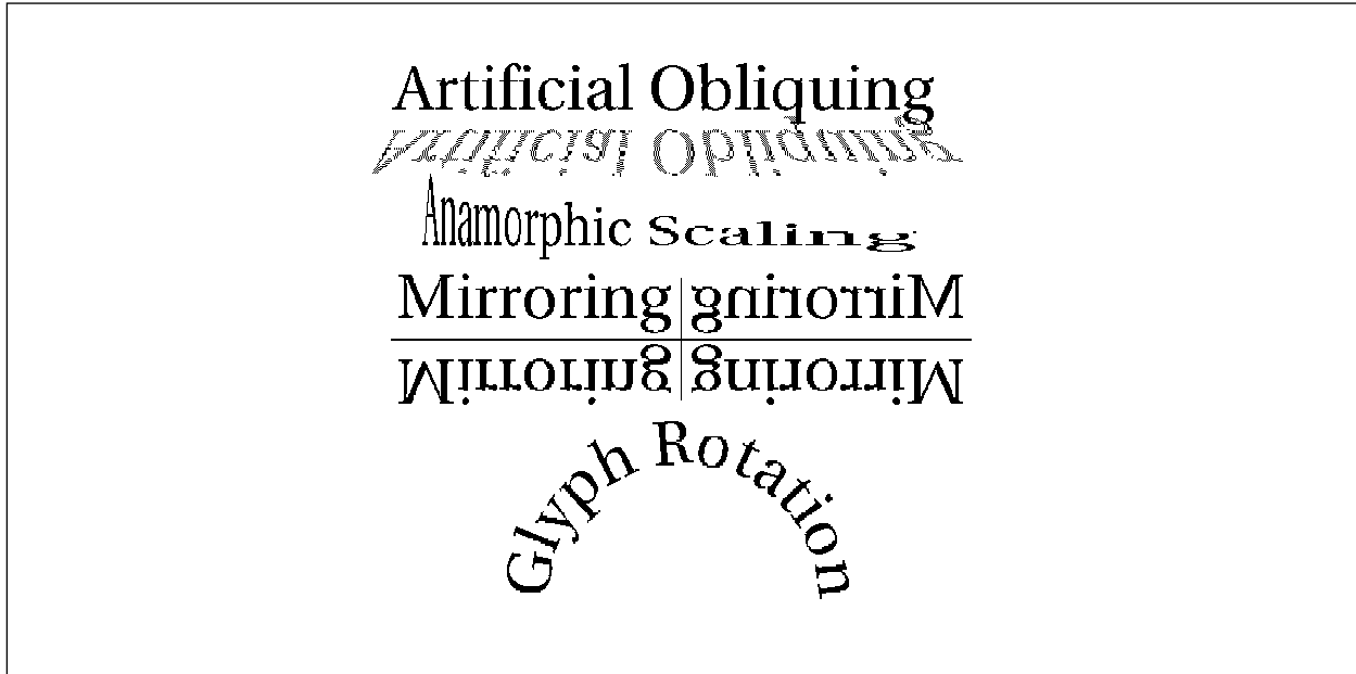
Figure 3: Some of the effects achievable with affine transformation matrices — all obtained from the same Adobe Utopia scalable font
