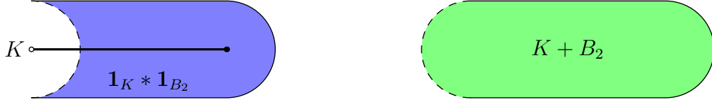
Figure 6.2: Let K be the half-open segment at left. The convolution function \mathbf{1}_K * \mathbf{1}_{B_2} has value one on the (non-compact) blue region and zero elsewhere. It is not the characteristic function of the Minkowski sum K + B_2 , which is depicted in green at right.
