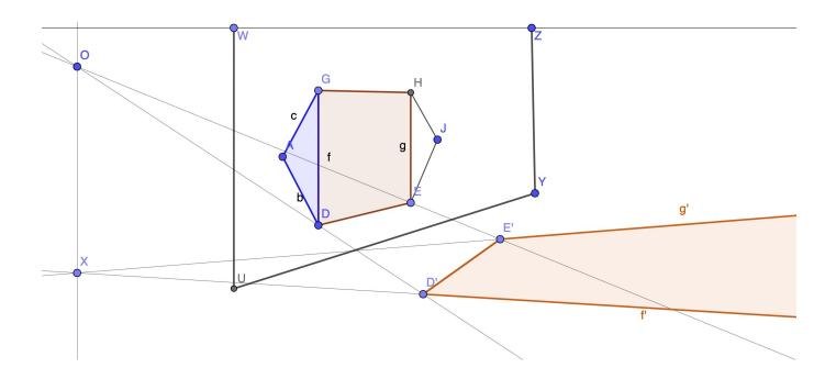
Let X denote the base of the lamp. The lamp stem OX is vertical, hence parallel to the wall. In particular it is parallel to segment f, hence in the plane  $\alpha$  determined by the point O and the segment f. The shadow f' is also in  $\alpha$ , and is in the plane  $\beta$  of the floor as well. Hence f' intersects the vertical line through O at X, in other words, to draw X, we can intersect the vertical line through O with the line f'.
