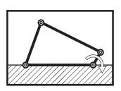
This linkage is used to transform spinning motion (from, say, a motor) into rocking motion (as in a windshield wiper). The configuration space of such a linkage is  $\mathbb{S}^1 \sqcup \mathbb{S}^1$ , the **coproduct** or **disjoint union** of two circles. The second circle comes from taking the mirror image of the linkage along the axis of its fixed rod in the plane and repeating the circular motion there: this forms an entirely separate circle's worth of configuration states.
